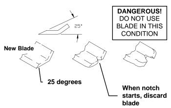
**C.** Sharpen blades with a hand file, electric grinder or blade sharpener. Wear gloves and eye protection when sharpening. Grind blade at original 25 degree bevel.
